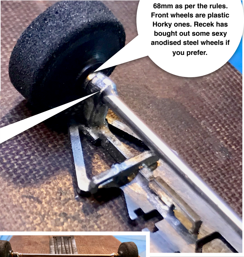
The piano wire axle is cut later to create two stub axles.
