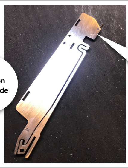
solder polished off by scrubbing on sand paper
