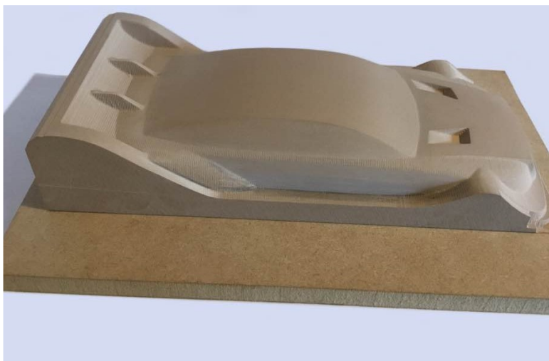
From this to this. Sandy cuts a mould for a vac formed body shell for Scuderia 66.
